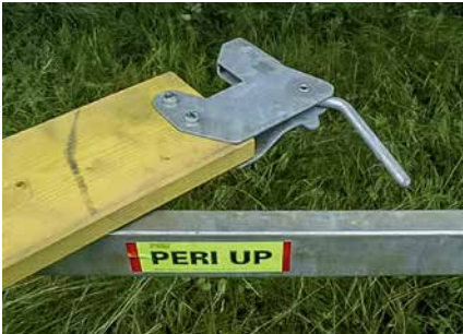
Toeboard Wood UPT ■ damaged metal fitting
