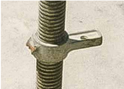
Spindles UJB / UJS / TR 38-70/50 ■ wingnut is defective
