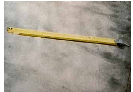
Toeboard Wood UPT ■ toeboard is broken
