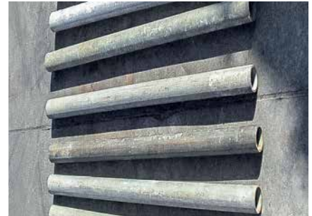
Scaffold Tubes ■ bent ■ no dents or buckling of the tube profile ■ permitted bending \leq L/200
