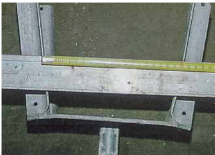
Cross Forkhead ■ bent head plate > 5 mm
