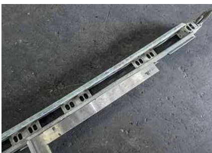
Ledger UVH ■ bent = steel deck cannot be mounted
