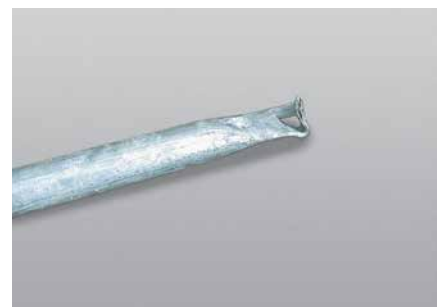
Guardrail UPG ■ bent ■ visible cracks ■ permissible angle deviation > 45°
