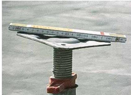
Spindles UJB / UJS / TR 38-70/50 ■ head or base plate is broken
