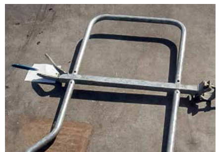
End Guardrail UPX ■ bent fork \leq 20 mm
