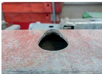
Ledger UH ■ opening is bent
