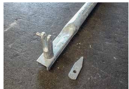
Ledger Brace UBL ■ missing gravity pin
