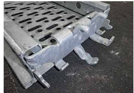
■ Scaffold Decks UDI / UDG ■ claw is bent or cracked
