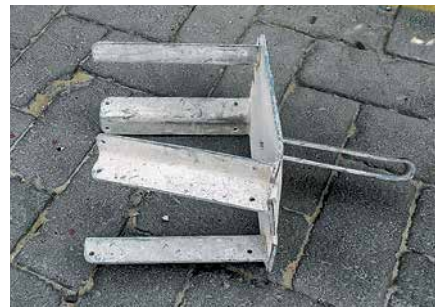
Crosshead ■ bent ■ bent and with crack on the welding seam ■ angle is damaged
