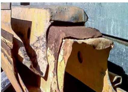
Toeboard Steel UPY ■ heavy deformation of the toeboard edges
