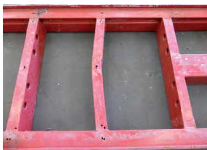
Kink in the perforated strut
