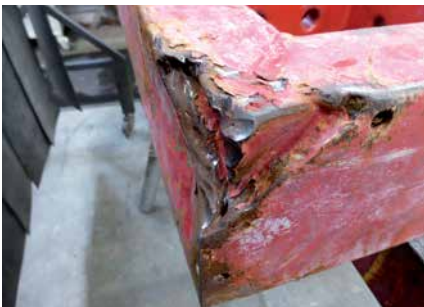
Levering corner deformed
