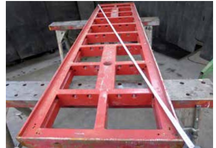
Element bent across the diagonal > 6 mm
