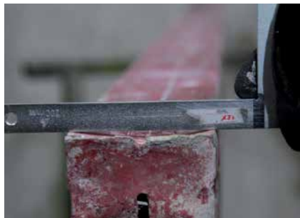
Dent in Wall Thickness Compensation > 3 mm
