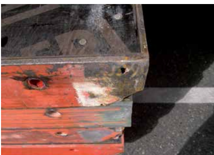
Holes in profile \leq \varnothing 3 \text{ cm}
